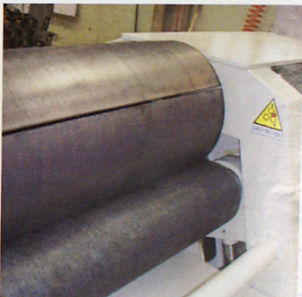
Figure 3 If the prebending is done correctly, the seam should come together nicely.
