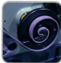
STANDARD Scroll Tool w/ Scroll Former and Fixed Bar Support.
